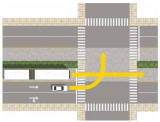
Figure 16 Center BRT lanes with mid-block crossing on a urban arterial (EMBARQ, 2012)
