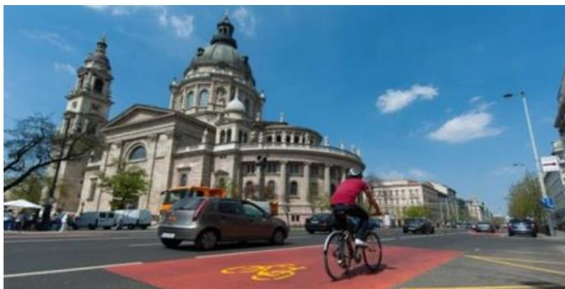
**Figure 18** Bike box with clear marking in Budapest (Transport Strategy BKK, Centre for Budapest Transport, 2015)
