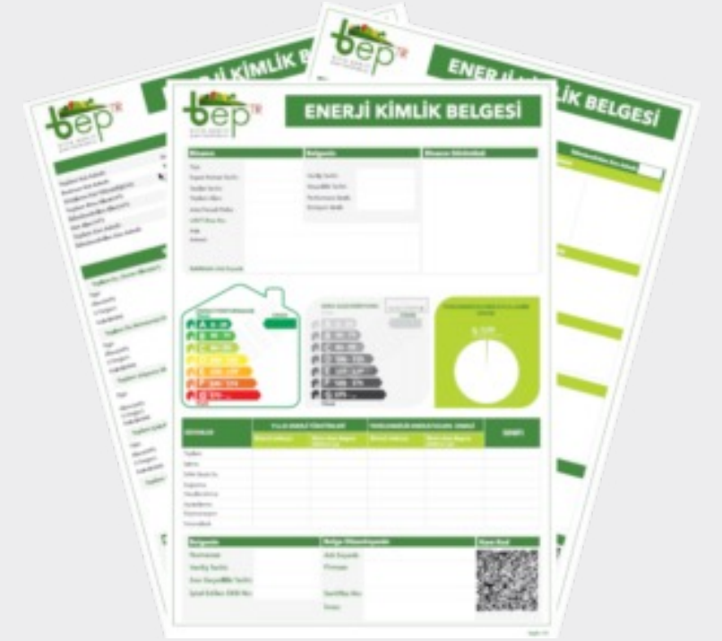
Figure 20. Energy Performance Certificate (EPC) issued to buildings in Türkiye through the BEP-TR system [84].
