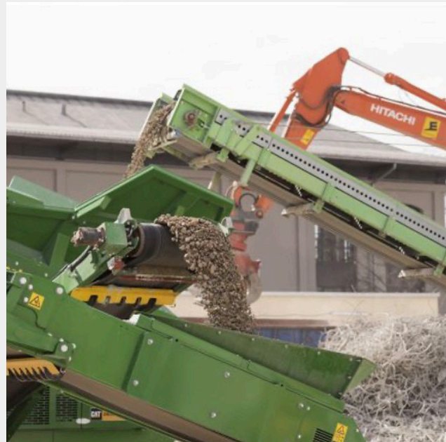
Concrete was cleaned and sorted on-site
