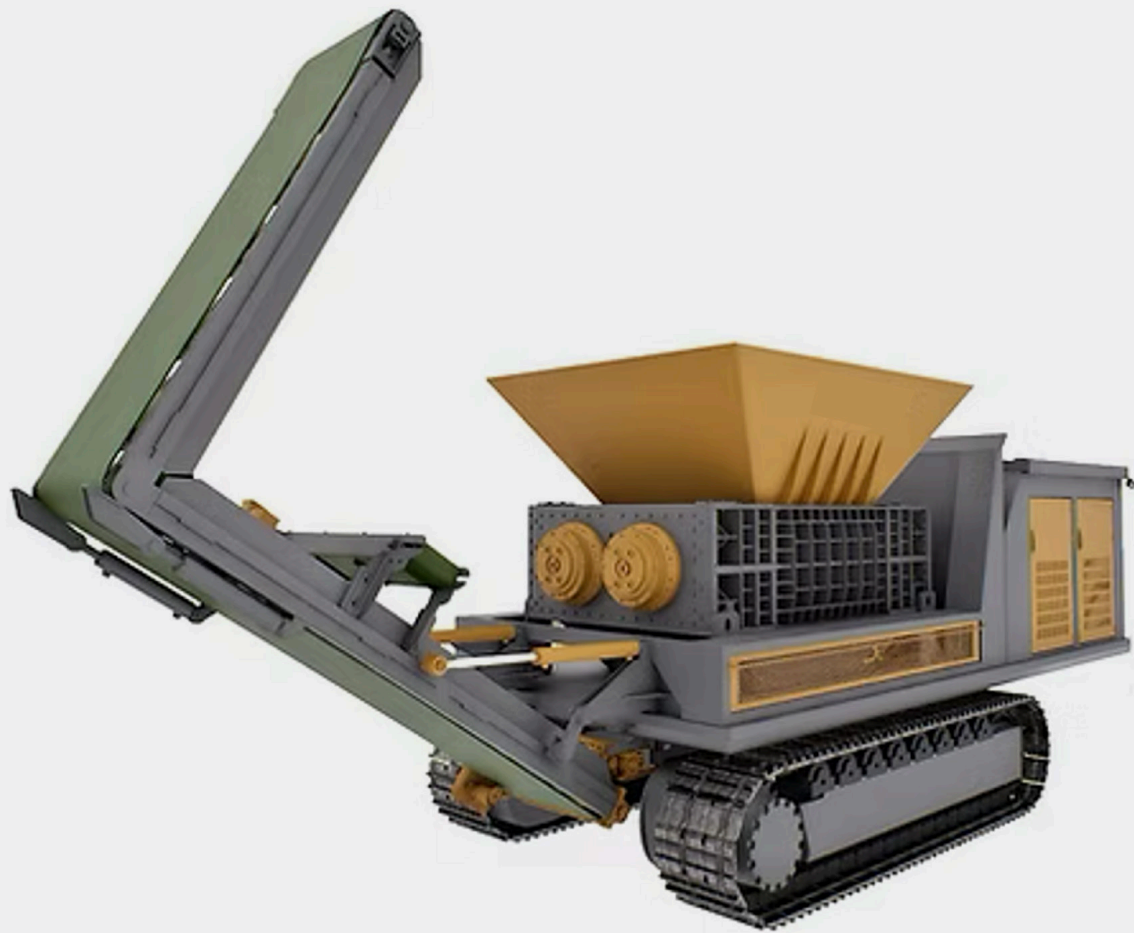
Image: On-site recycling technologies are rapidly advancing. The image shows a mobile crusher performing on-site concrete recycling [17].
