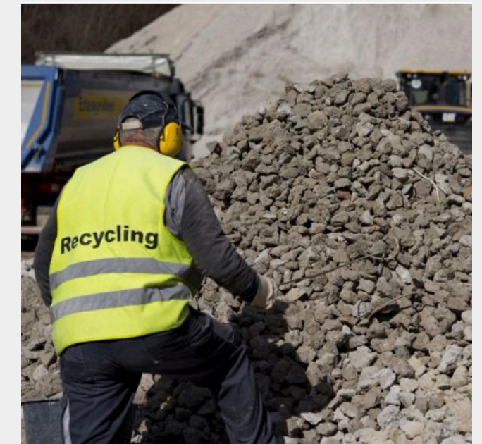
Concrete was used as road fill material.
