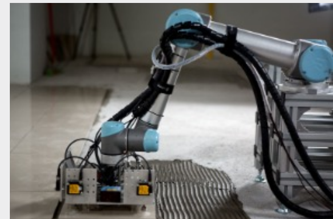
Tile-laying Robot © Gramazio Kohler Research, ETH Zurich
